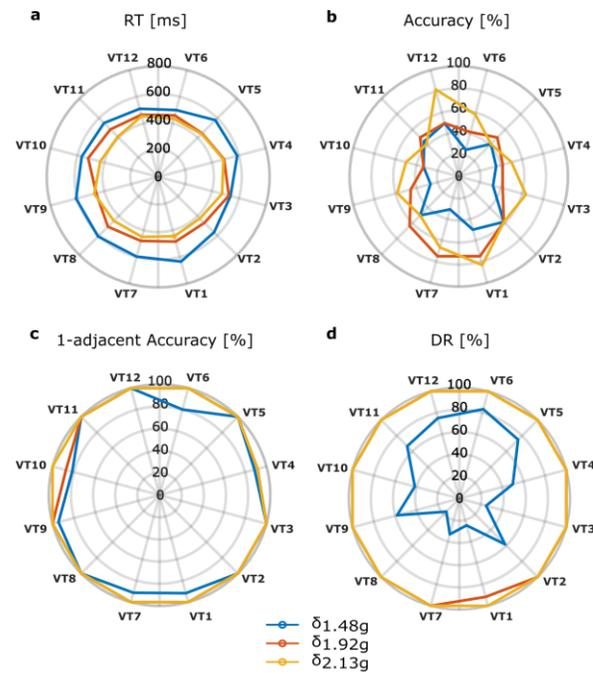
Fig. 3 Spatial distribution of (a) RT [ms], (b) Accuracy [%], (c) 1-adjacent Accuracy [%] and (d) DR [%] around the waist, at the twelve locations where VT units were placed. Data are aggregated across subjects, with values indicating medians.
