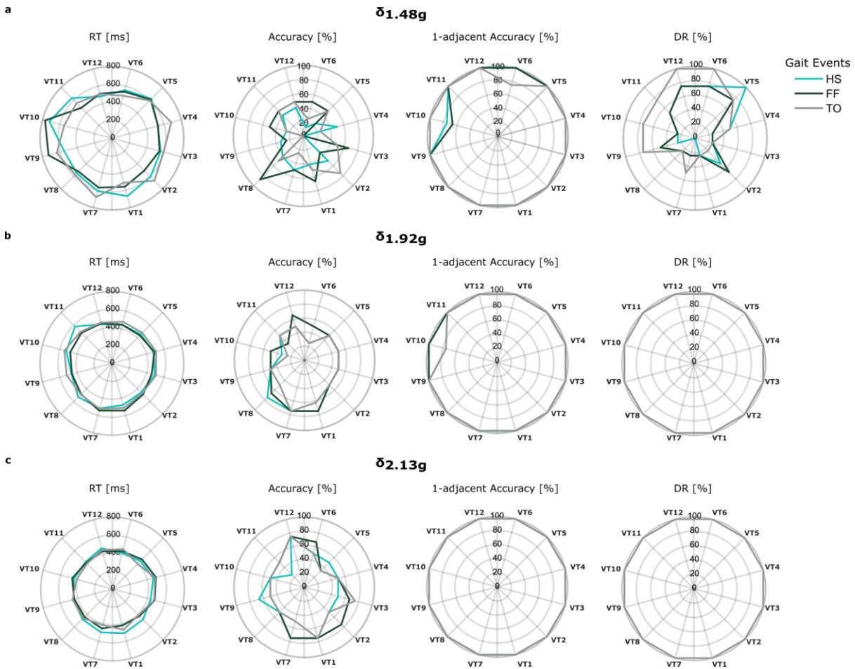
Fig. 4 Spatial distributions of RT, Accuracy, 1-adjacent Accuracy and DR calculated for each gait event (heel-strike, HS, foot-flat, FF, and toe-off, TO) at (a)  $\delta_{1.48g}$  (b)  $\delta_{1.92g}$  and (c)  $\delta_{2.13g}$ . Data are aggregated across subjects, with values indicating medians.
